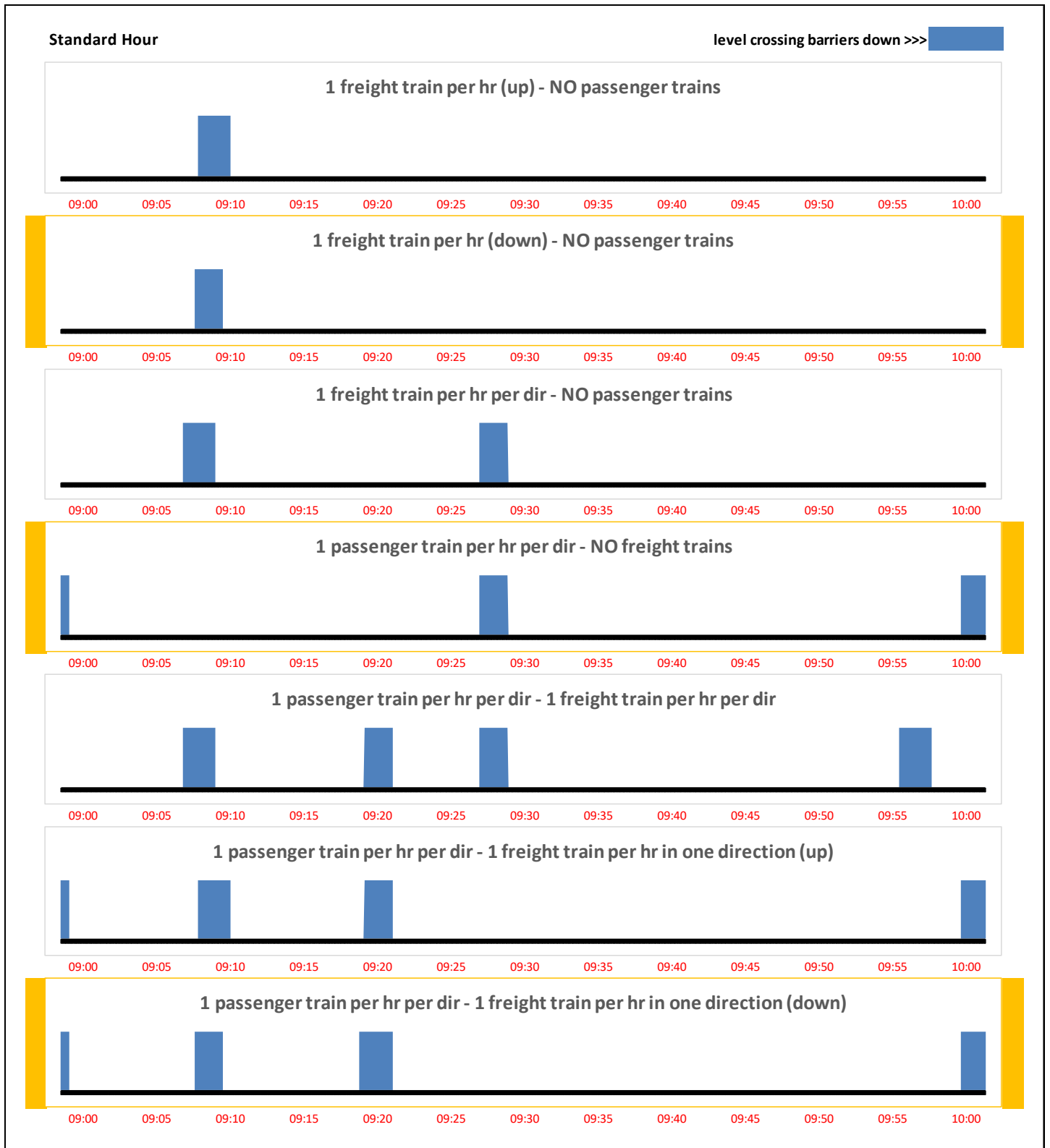
Figure 3: Ashton Vale Road Level Crossing closure times in a standard hour (chart) Source: based on 'Concept Trains Plans for Various Scenarios 0.3.xlsx' with revised level crossing closure times supplied by NR
